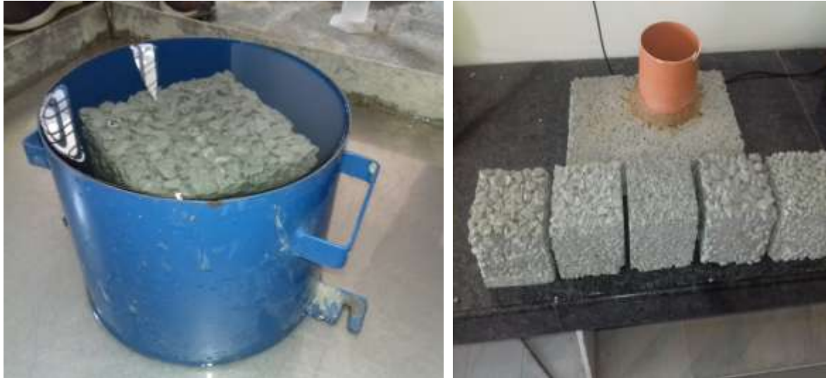
Fig.1 Casting & testing of Pervious concrete in lab
